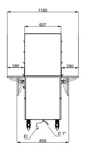
D = Drain El = Electrical inlet (power)
